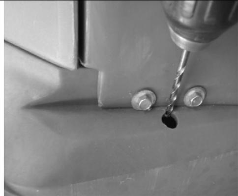
**8)** Drill out dimples on **inside** of base runners in **front** (1left runner & 1 right runner) using a 1/2" dia. drill bit. Drill directly on top of 1/2" hole using 3/16" drill bit & 3/16" hole should be open into 1/2" hole. Base PN 19015(roto-mold).
