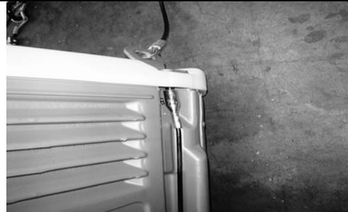
**6)** Drill out dimples on **outside** of base runners in **front** (1left runner & 1 right runner) using a 1/2" dia. Drill bit. Drill directly on top of 1/2" hole using 3/16" drill bit & 3/16" hole should be open into 1/2" hole as shown below. Base PN 19015 (roto-mold).
