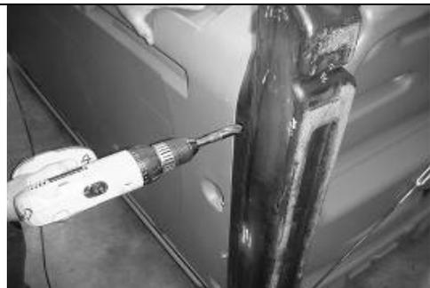
**12)** Thread male end of cable through drilled holes in runner from outside to inside. Once cable is through runner it should fit 3/16" holes drilled in runner.
